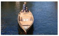
Kawasemi Cargo boat Length 7.73m Width 1.36m Depth 0.40m Passenger 4 Boat man 2 Total 6
